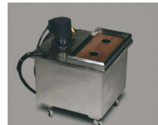
Recirculating Cooling Unit
