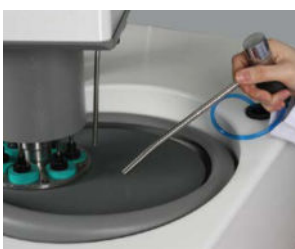
Retractable water hose for easy cleaning
