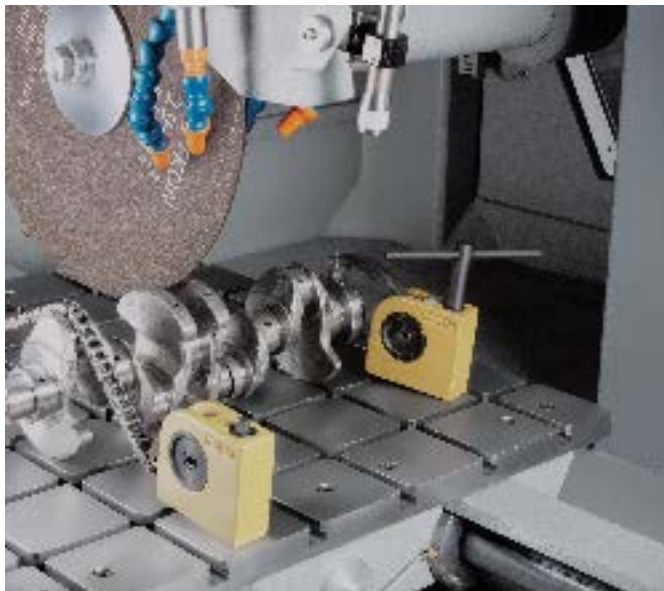
Extra large cutting chamber with easy access and handling.
